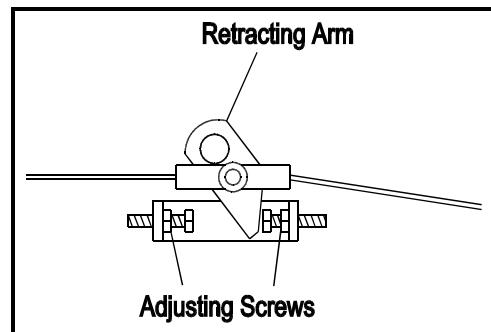
3. The final step is to ensure that the Track Parking Brake is functioning correctly. It is designed to stop and hold rated load on the stairway. To do this, the Brake Spring must pull on the Brake Mechanism without any resistance from the Brake Cable. This can happen if the Front Brake Cable does not have sufficient slack.
