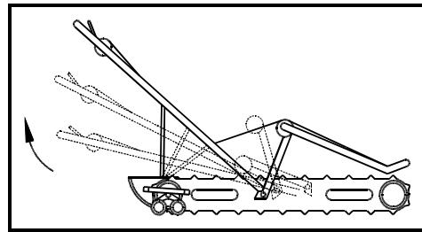
2. Ensure Evacu-Trac is properly locked in the open position. Check the Indicator Window on the side of the aluminum track frame. If it is **blue** the seat is properly locked.
