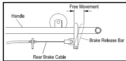
The Brake Release Bar travel range is adjusted using the Adjusting Screws that control the Front Auxiliary Wheel Retracting Arm. Loosen the lock nuts and adjust as required. Test the action of the Brake Release Bar and then tighten the lock nuts.
