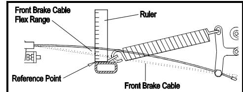
Adjust the cable as required using the Adjusting Nut on the Brake Actuation Arm. Tighten the Adjusting Nut and test the function of the Brake. It should stop and hold Evacu-Trac on the stairway with rated load. It should also release fully when the Brake Release Bar is squeezed all the way back to the handle, allowing Evacu-Trac to descend the stairway at a comfortable speed, as shown in the Training Video.
