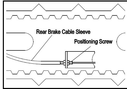
2. When you squeeze the Brake Release Bar it should travel until it just makes contact with the lime green Handle. This will allow you to comfortably hold Brake Release Bar in its released position when pushing Evacu-Trac on flat surfaces or descending a stairway.
